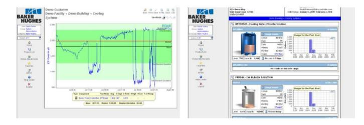
The Web Browser option is a good tool in locations where there are concerns about installing software on the plant computers. The Web browser option allows you to connect to the controller to view live data, acknowledge alarms and change settings.
